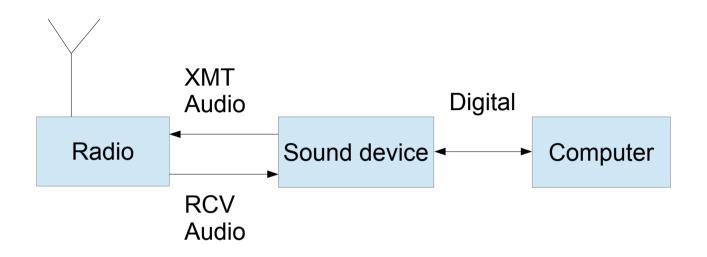
**Radio** – HF Rig, VHF, HT, etc. (xmt/rcv audio and PTT)
