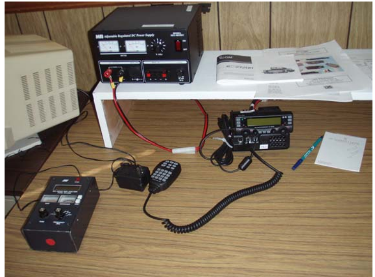
Dual band radio with Ed’s well-traveled antenna analyzer
