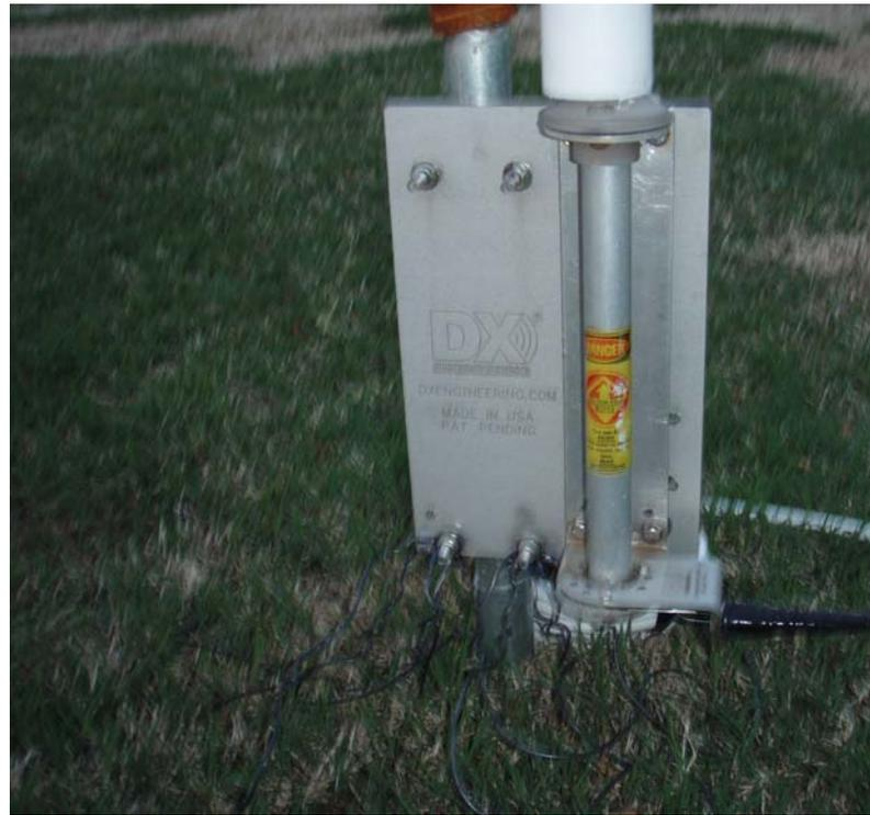
This picture shows the base with the radials connected.
